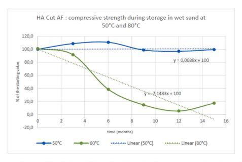
With the equations of both trend lines the time for the compressive strength to drop to 80 % of the starting value can be calculated. The following Arrhenius plot can be made by putting the temperatures in 1/K \* 1000 and taking the logarithm of the time in hours.
